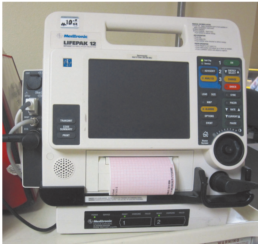
Figure 1-5 A portable ECG monitor is transported to the scene during a cardiac emergency and is attached to the patient. The ECG tracing is recorded and viewed by the emergency personnel. In addition, the tracing can be transmitted to the hospital, where a physician can evaluate and determine the necessary drugs and treatment for the patient based upon the heart rhythm viewed and the report from the emergency personnel.
