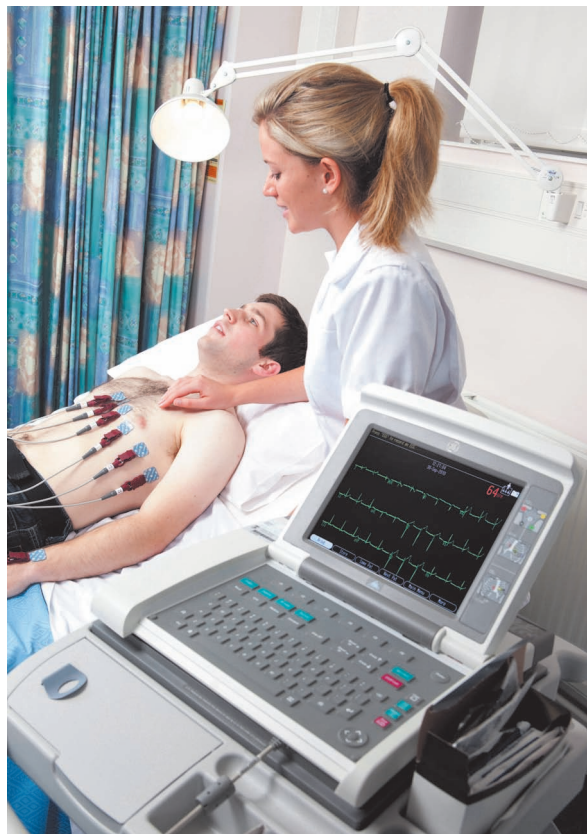
Figure 1-1 Today's 12-lead ECG machine is attached to the patient's chest, arms, and legs using electrodes and lead wires. It records a tracing of the electrical activity of the heart.
